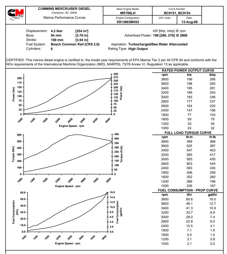
Rated Conditions: Ratings are based upon ISO 8665 and SAE J1228 reference conditions; air pressure of 100 kPa [29.612 in Hg], air temperature 25deg. C [77 deg. F] and 30% relative humidy. Power is in accordance with IMCI procedure. Member NMMA.
